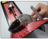
▲ Clubhead soling plate provides precise postioning for measuring lie and loft angle as well as face procgression on woods, irons and putters
