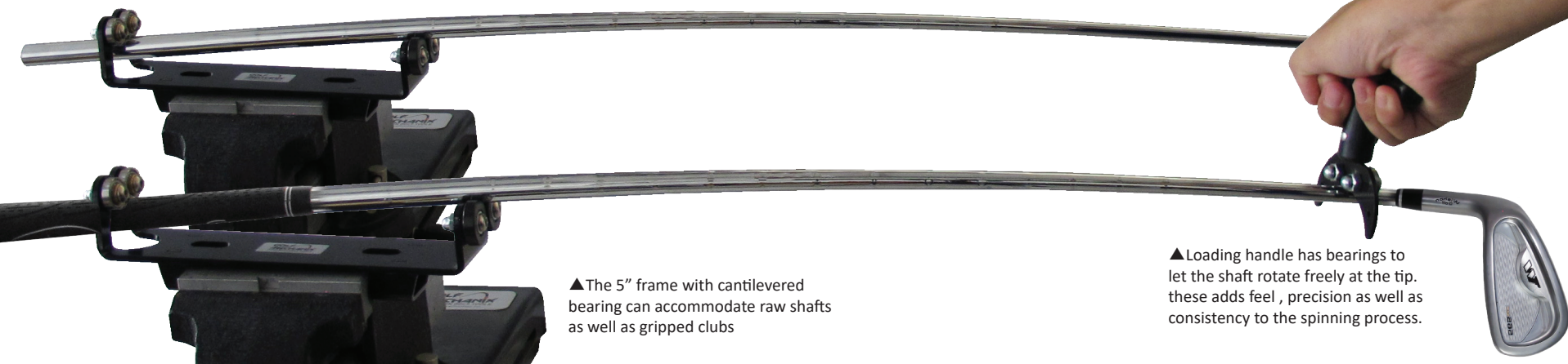
▲Forward mounted sheaves are capped with a tough engineering plastic that protects the shaft structurally as well as cosmetically.
