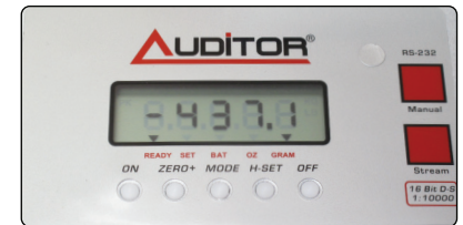
▲ Measures total weight of clubs & components to 0.1 g accuracy.
