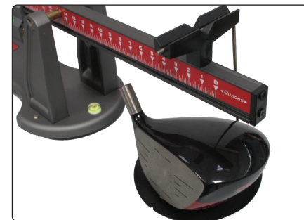
▲ Weighing club components in both grams and ounces to industry standard tolerances.
