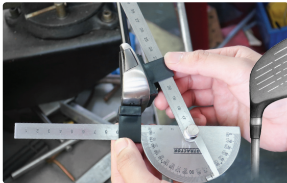
▲ Measuring Loft Angle
