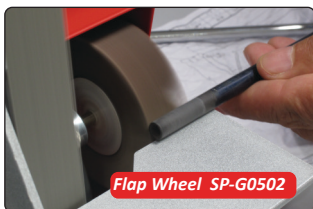
▲ Flap wheel removes thin film coatings off graphite shafts
