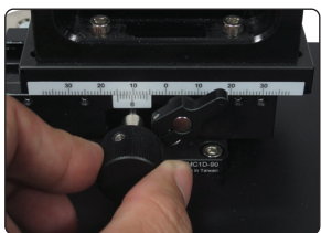
▲ Micro-metric slide places the club face slide accurately in relation to the impact ball.
