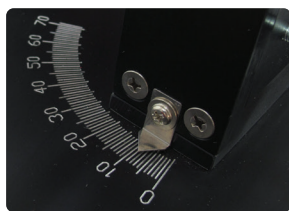
▲ Tower can be de-lofted to allow all clubs including irons and hybrids to be tested effectively.
