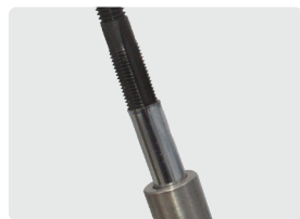
▲ Cut thread into broken shaft to a sufficient depth
