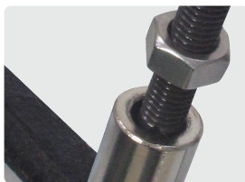
▲ Slip extender over the tap and screw the nut on
