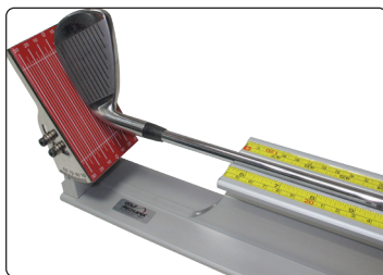
▲ “Deep throat” provides sufficient clearance to accommodate back of heel geometry of any club, putters fitted with double bent shafts, belly putters, and putters fitted with oversized jumbo grips.
