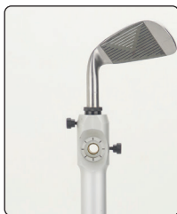
▲ Multiple axes of rotation planes for building inertia matrixes
