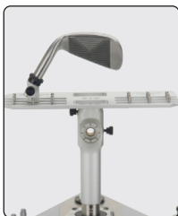
▲ Setup for measuring MOI to R&A specifications
