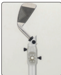
▲ Multiple axes of rotation planes for building inertia matrixes
