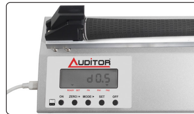
▲ Swing weight is displayed in 0.5 SW point increment
